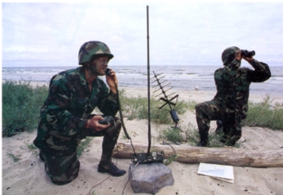
The Harris AN/PRC-117F radio was originally developed for U.S. Special Forces to provide ground-to-ground, ground-to-air, and ground-to-satellite secure communications in one radio package.
