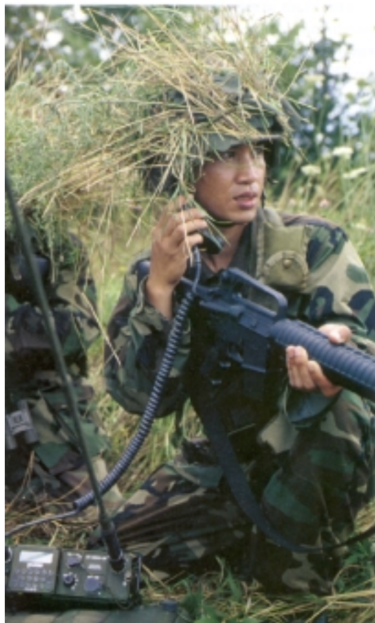
Soldiers use the RF-5800H-MP to provide long-range HF voice and data communications.
